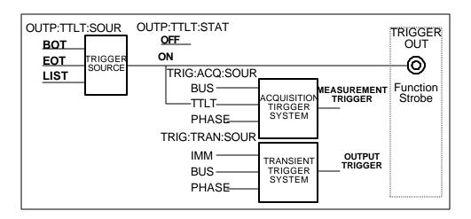
Figure 6-5 : Trigger system block diagram
