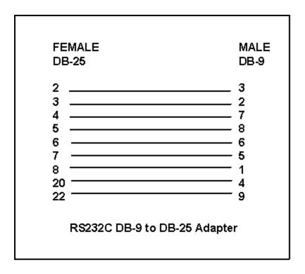
Figure 3-2 : DB9 to DB25 Adaptor Wiring Diagram
