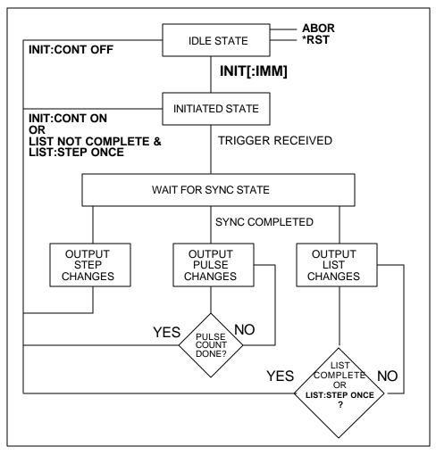
Figure 6-2 : Transient Trigger System Model
