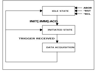
Figure 6-3 : Measurement Acquisition Trigger Model
