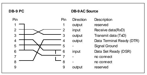
Figure 3-1 : RS232C Interface Cable Wiring Diagram
